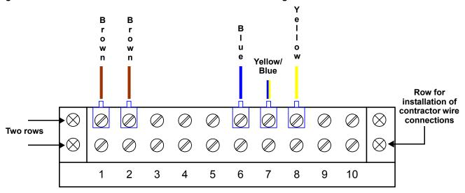
The recommended gauge for status/control connection wires is 16 AWG - 600VDC (1.3mm<sup>2</sup> wire section). Status/Control wires must be sized and installed in compliance with all applicable local, regional and national regulations (e.g., National Electric Code for USA).
